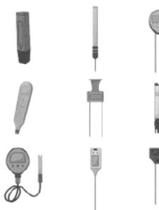
A thermocouple thermometer measures temperature using two different metal wires. Both wires must touch a surface to measure its temperature. This thermometer finds temperature by measuring the flow of electricity between the wires and is extremely accurate. Some are used to measure body temperature, while others are used for measuring the temperature of liquids and food. There are also thermocouple thermometers that can measure over 1,000 degrees, so they are commonly used in factories.
