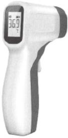
Infrared thermometers measure body and surface temperature using infrared light sensors. They are usually held in the hand and do not need to touch something to measure its temperature. Infrared thermometers work very quickly, so they are useful for measuring the body temperature of small children. However, they can be easily affected by the heat of other things, such as the temperature of the air, sunlight, and thick clothing, so they are not very accurate.
